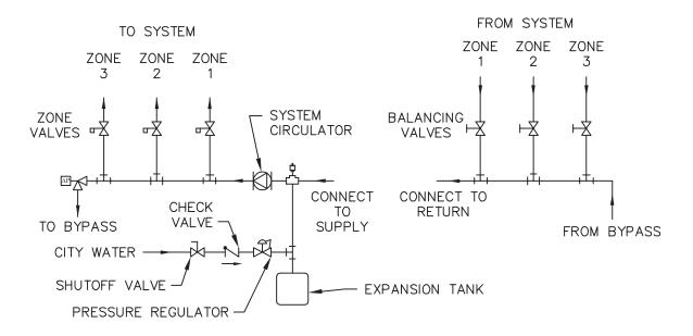
Figure 3.5: Zone Piping with Zone Valves
